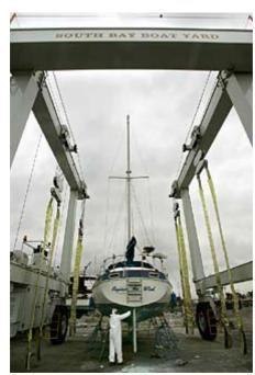
This 100-ton lift will be something of a lightweight when a new crane – billed as the largest of its kind – arrives at the South Bay Boat Yard. The new one can hoist more than 600 tons.
