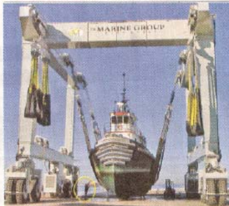
Marine Group's new Travelift hardly breaks a sweat lifting this harbor tug. Note the size of the guy (circled) powerwashing the bottom.
