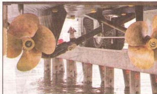
A worker directed the movement of the company's new Travellift as it raised the 193-foot mega yacht out of a slip.
